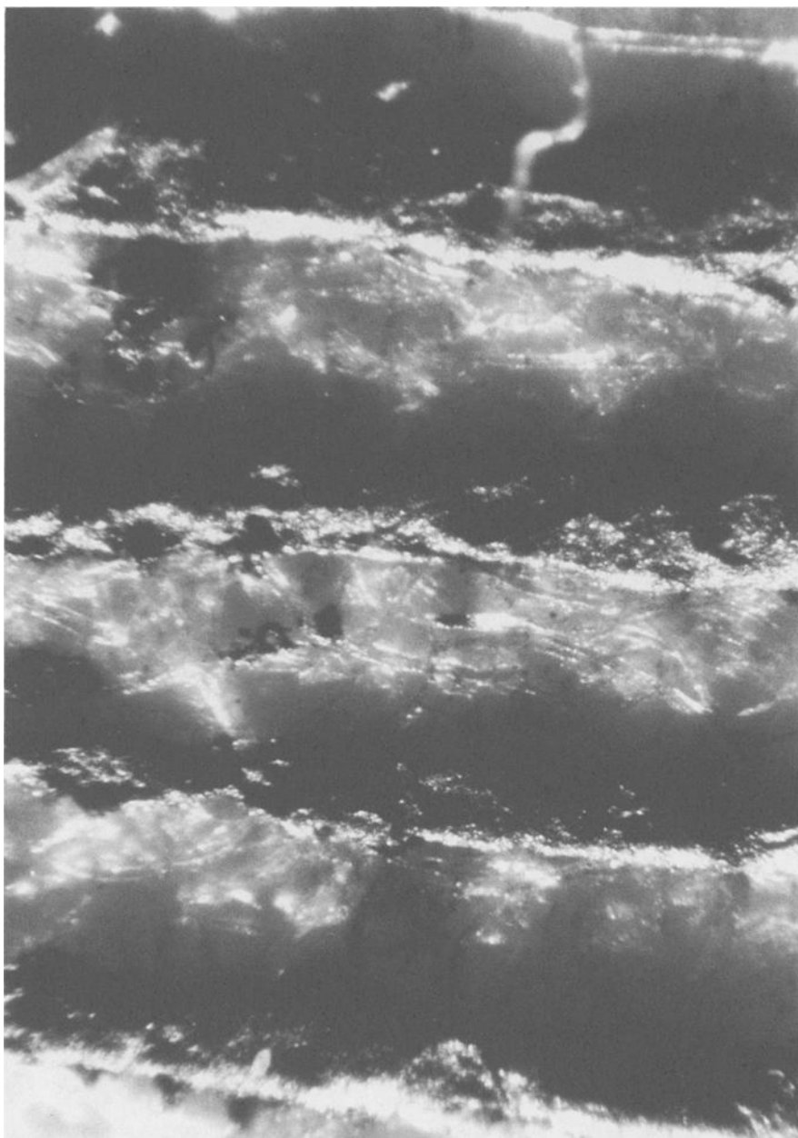
FIG. 7—Intaglio magnified shows the shadow left of the image lines that are embossed on the paper opposite the light source from the right side.
