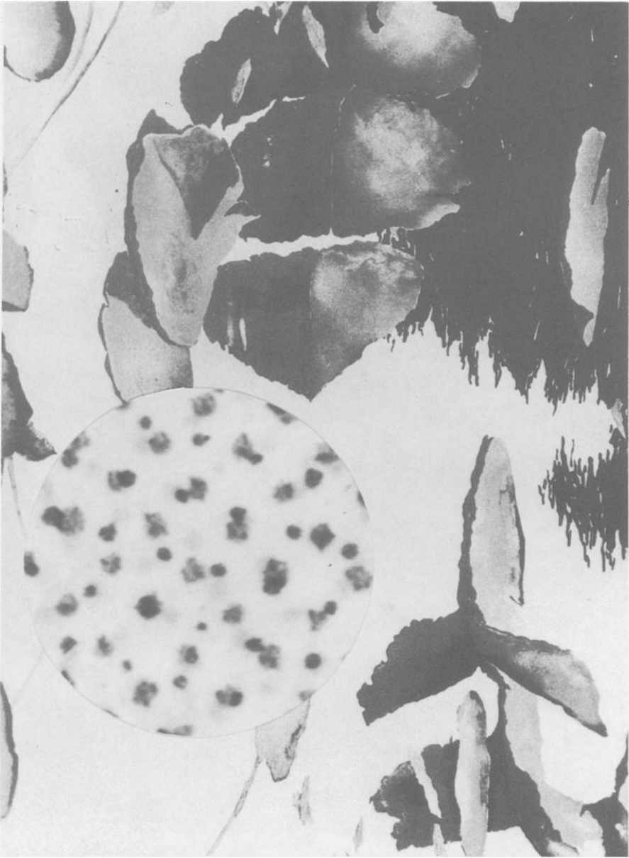
FIG. 6— Photomechanical lithograph with an enlargement of the dot matrix represented in circle.
